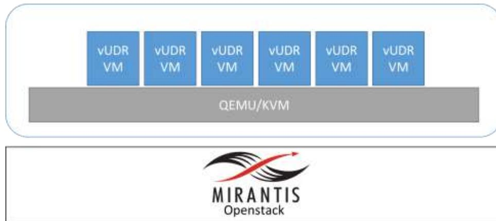
Figure 3 - vUDR Deployment on Mirantis OpenStack
